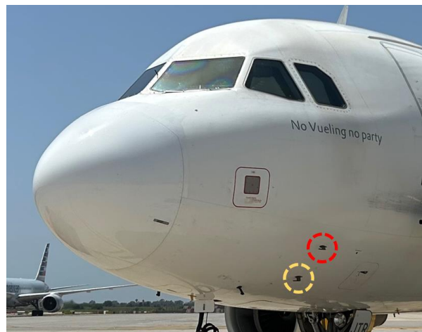
Figure 7: Location of the PITOT CAPT and PITOT STBY probes, highlighted in red and yellow, respectively.
