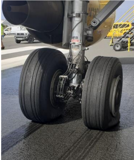
Figures 16 and 17: Condition of the main gear wheels after the incident. Figure 16 (on the left) shows wheels 1 and 2, and Figure 17 shows wheels 3 and 4.
