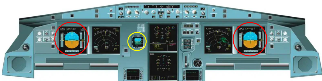
Figure 9: Location of the 3 anemometers on the EC-JTR aircraft. The captain's (on the left) and co-pilot's (on the right) PFDs are shown in red and the standby instrument in yellow.
