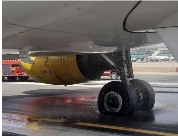
Figures 16 and 17: Condition of the main gear wheels after the incident. Figure 16 (on the left) shows wheels 1 and 2, and Figure 17 shows wheels 3 and 4.
