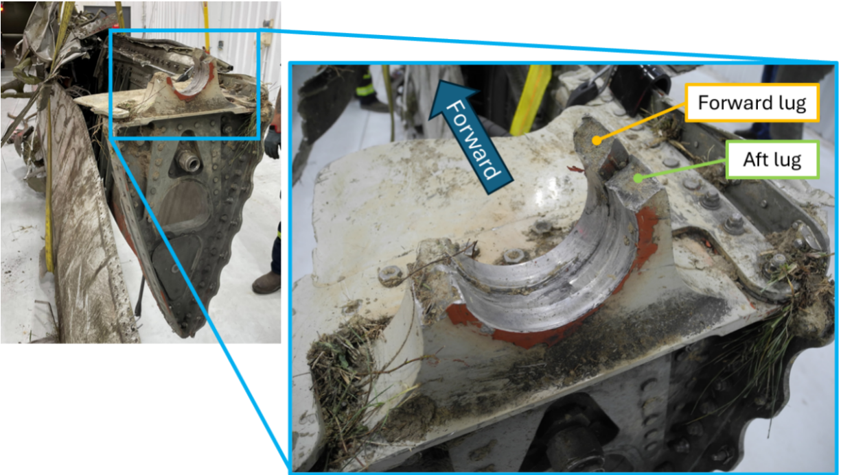
Figure 7. The separated left pylon after recovery (left image) and the left pylon aft mount's fractured forward and aft lugs (right/enlarged image).
