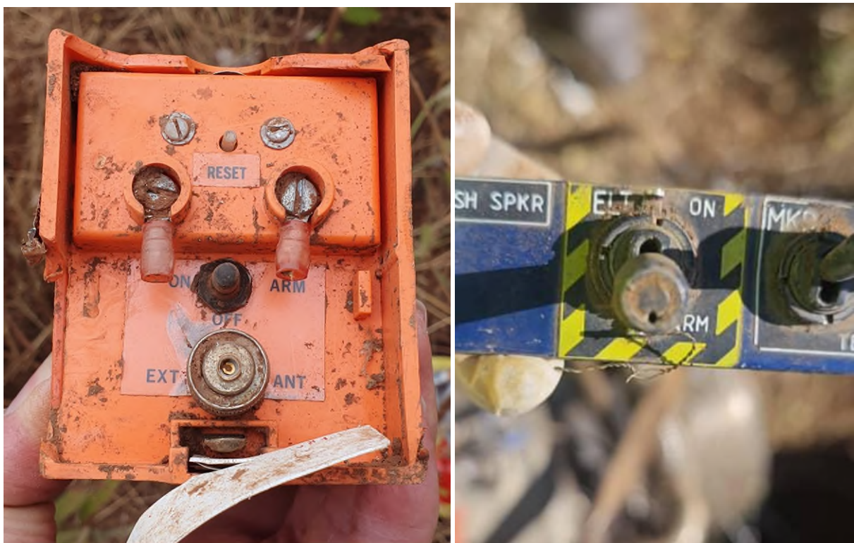
Fig. 11: Switch on the ELT in position 'OFF' (left), switch in the cockpit in position 'ARM'
