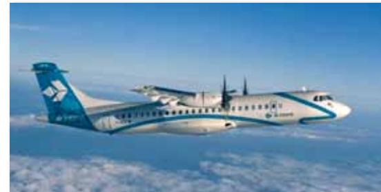
The ATR 72 is derived from the ATR 42 with a 4.5 m stretched fuselage. The two aircraft feature a high degree of commonality: the same cross section, the same cockpit for cross-crew qualification. Offering a standard capacity of 66 seats, the ATR 72-200 is equipped with two PW124B engines, rated at 2,400 SHP each. The derivative version of the basic ATR 72, the ATR 72-210 is equipped with two higher power 2,750 SHP PW127 engines.
