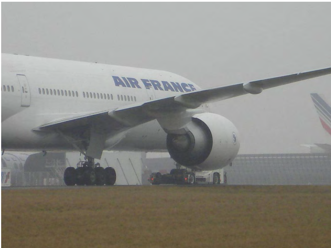
Figure 16. Engine Nacelle Blocking the Warning Lights
