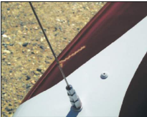
Figure 18-7. A string simply tied near the nose of the gyroplane that can be viewed from the cockpit is often used to indicate rotation about the yaw axis. An inclinometer may also be used.
