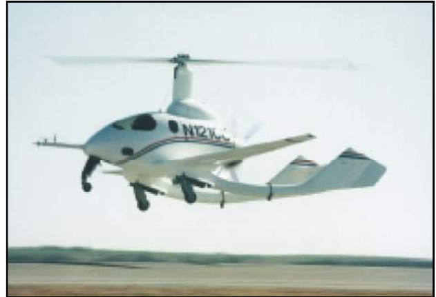
Figure 15-3. The CarterCopter uses wings to enhance performance.
