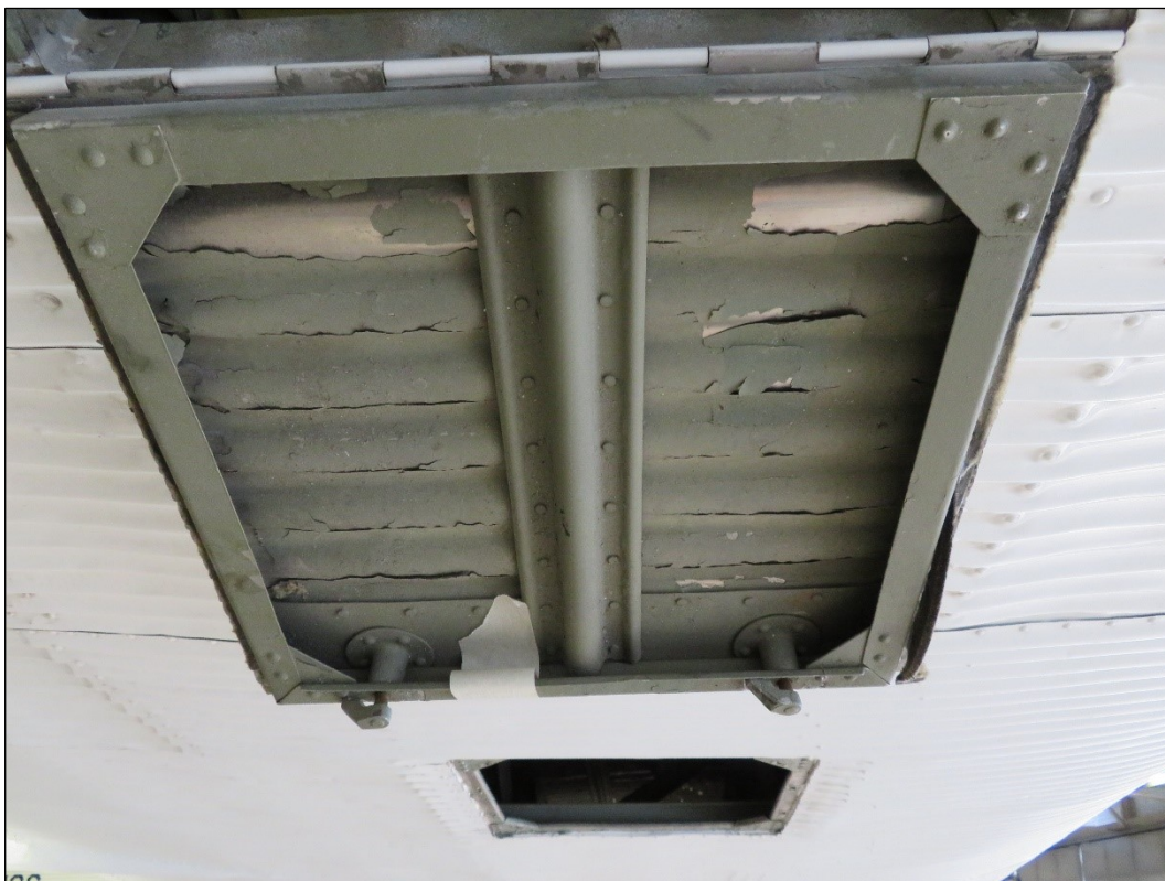
Figure 67: Surface flaking and a lack of anti-corrosion paint on the inside of HB-HOS's right-hand outer wing.
