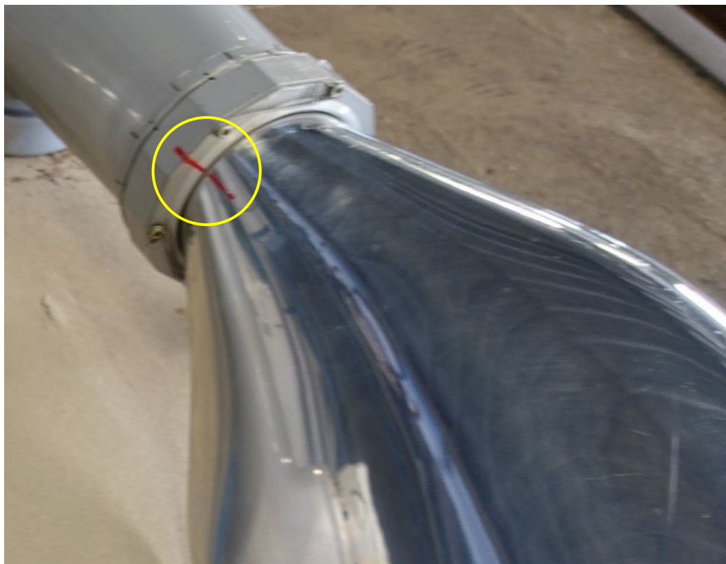
Figure 37: Red marking on the twelve-point nut and propeller blade (yellow circle).
