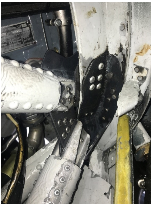
Figure 47: Remanufactured and assembled plate. Photograph provided by Ju-Air.
