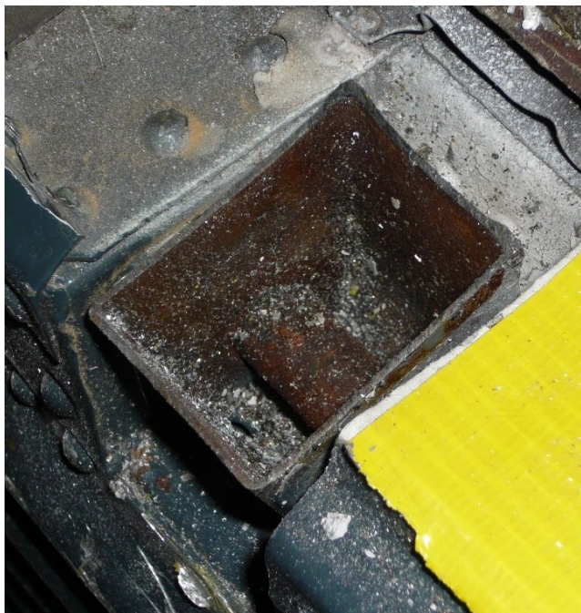
Figure 3: Close-up of figure 2 number (1) – severely corroded hinge of the cargo door on the right-hand side of the fuselage.
