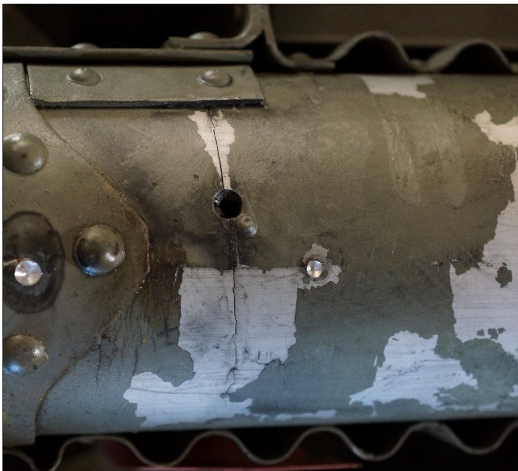
Figure 50: Exterior view – crack in lower spar I of the centre wing. Photograph provided by Ju-Air.
