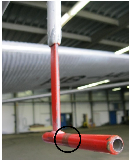
Figure 26: Pitot tube of HB-HOT. The openings for the static pressure are circled in black.
