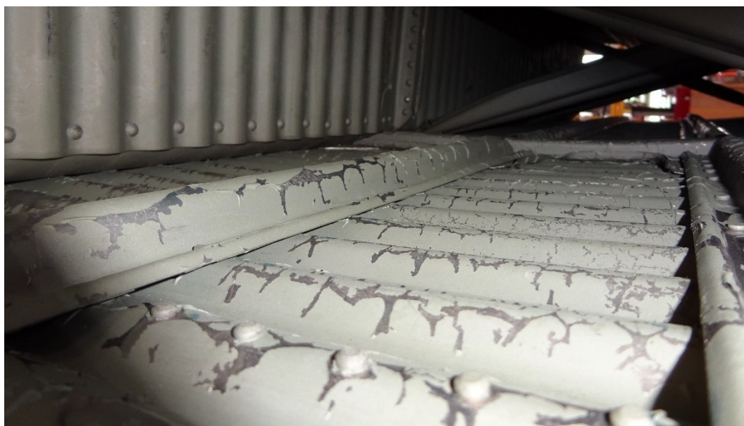
Figure 15: Inside of the horizontal stabiliser – areas where the anti-corrosion paint had partially flaked off.
