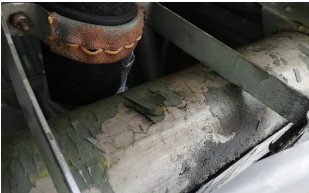
Figure 69: Lack of anti-corrosion paint on a spar tube in HB-HOP's left-hand outer wing.
