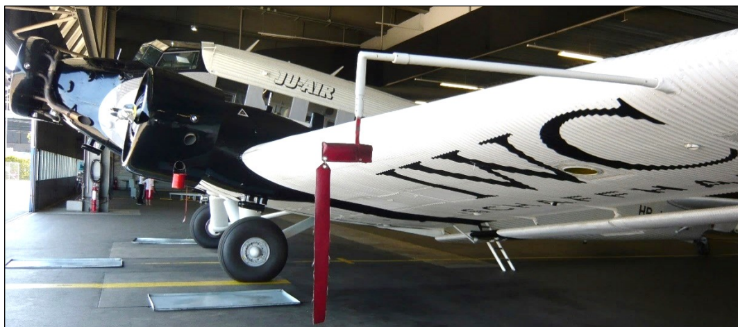
Figure 25: Arrangement of the pitot tube with red cover on sister aircraft HB-HOS.
