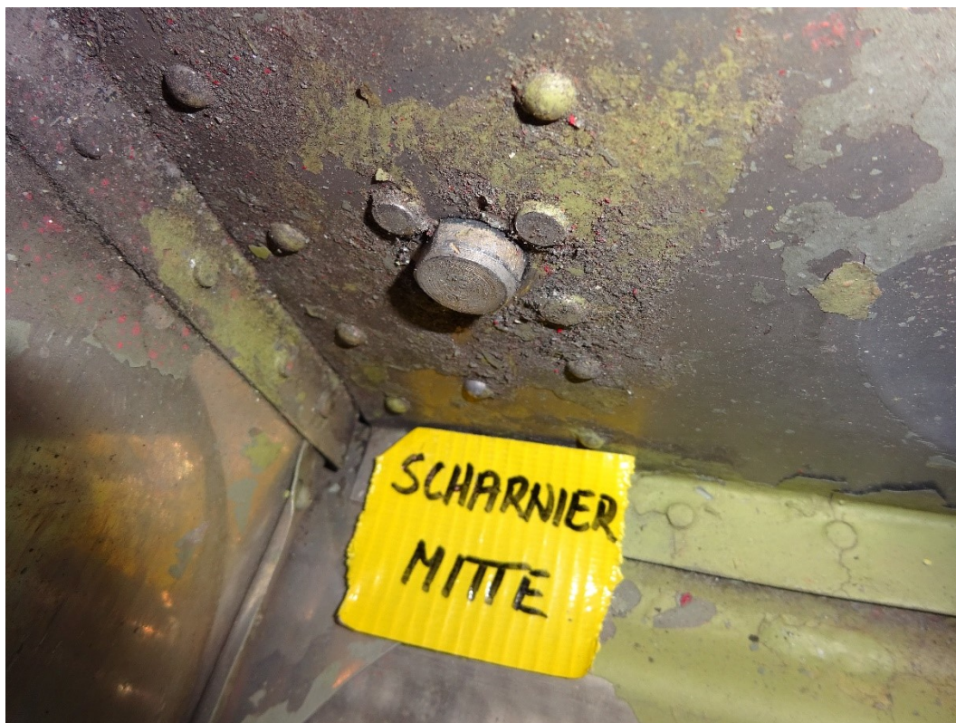
Figure 17: Inside of the rudder – head of the bolt for attaching the central hinge; lack of anti-corrosion paint; corrosion on sheet metal, rivets and bolt (label text reads central hinge).
