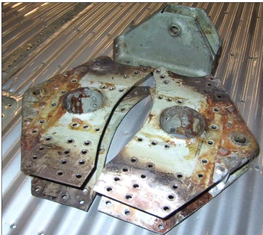
Figure 53: Removed, severely corroded components from the horizontal stabiliser. Photograph provided by Ju-Air.
