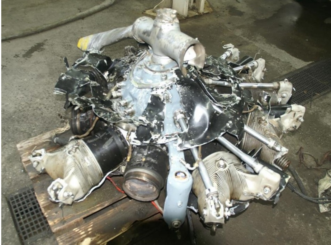
Figure 24: Engine cleaned using dry-ice blasting.
