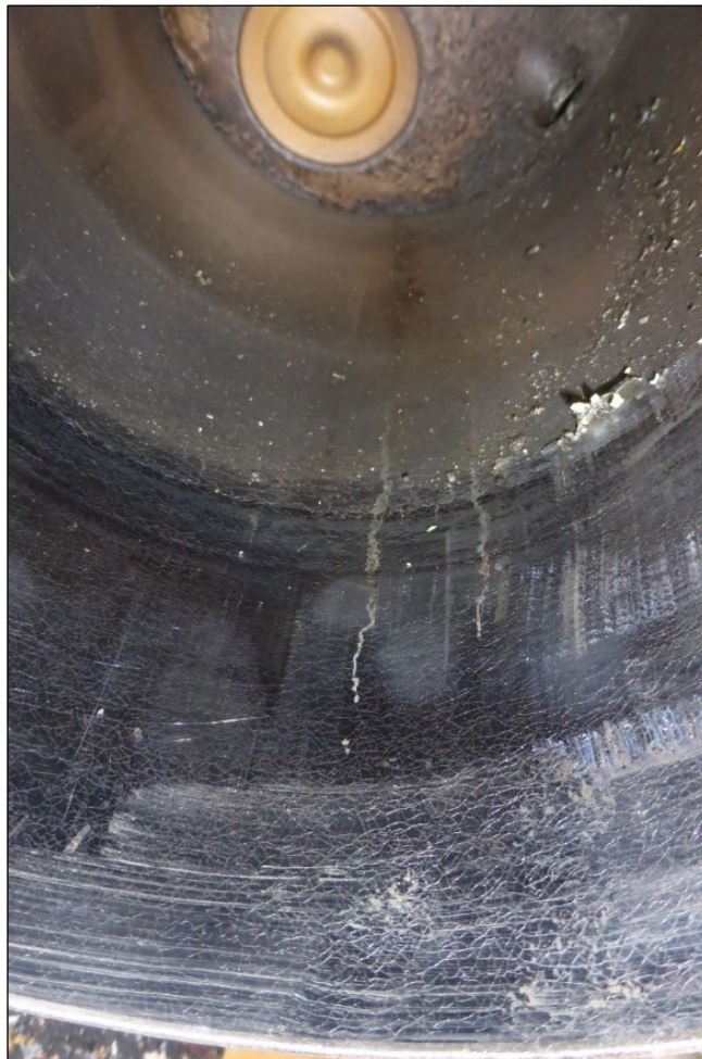
Figure 59: Example of a chrome-plated cylinder bore. The crack network typical for this method is clearly visible.
