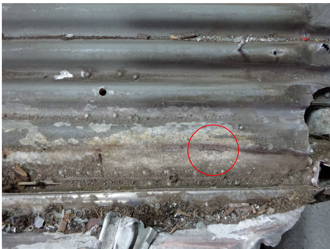
Figure 6: Close-up of figure 2 number (4) – severely corroded floor structure with fracture (red circle).
