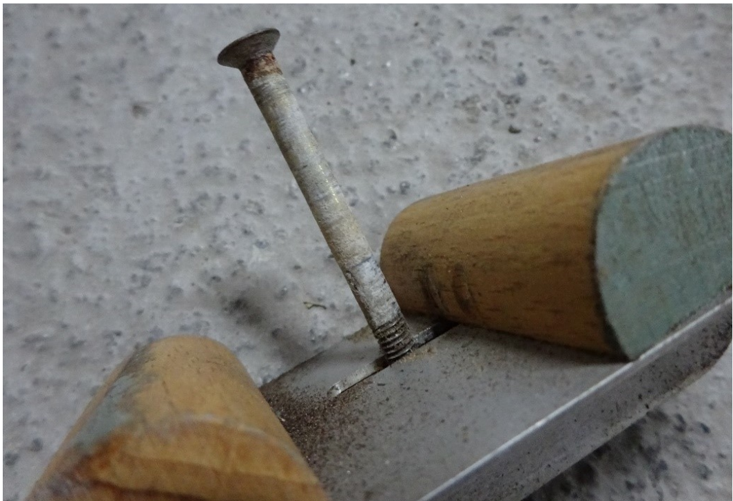
Figure 8: Severely corroded bolt for mounting a seat rail.
