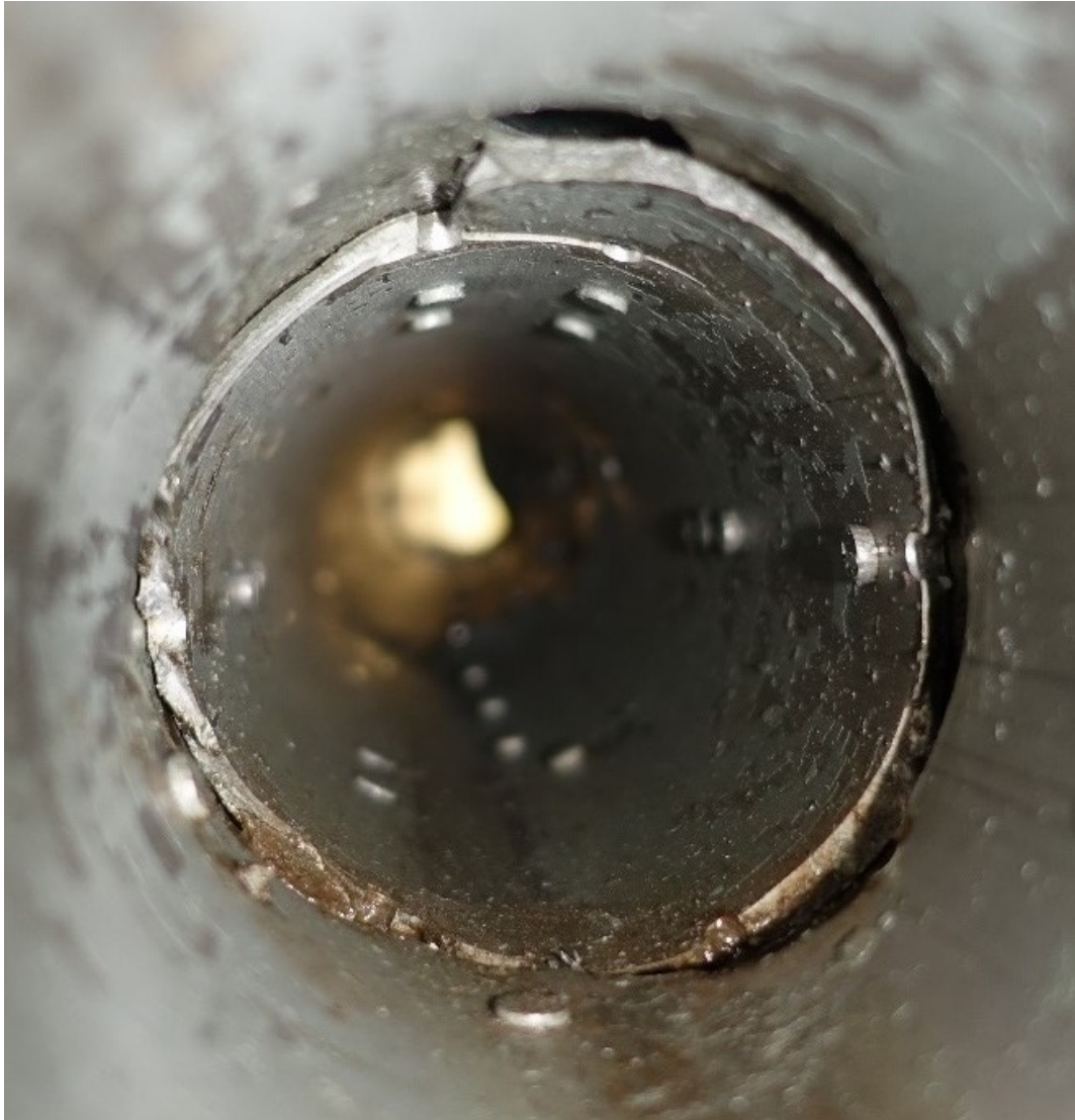
Figure 13: Close-up of the inside of the spar tube where fractures were found.
