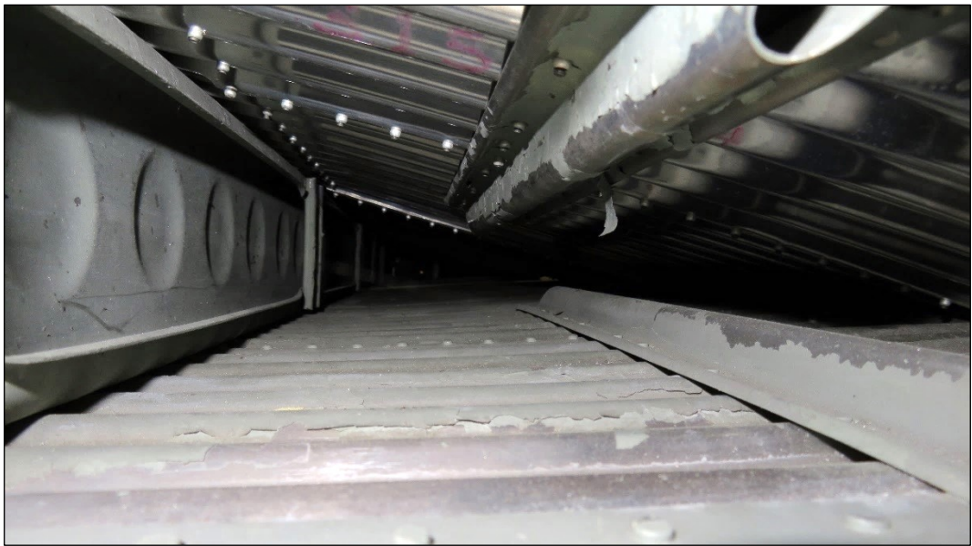
Figure 66: Surface flaking and a lack of anti-corrosion paint on the inside of HB-HOS's left-hand horizontal stabiliser.
