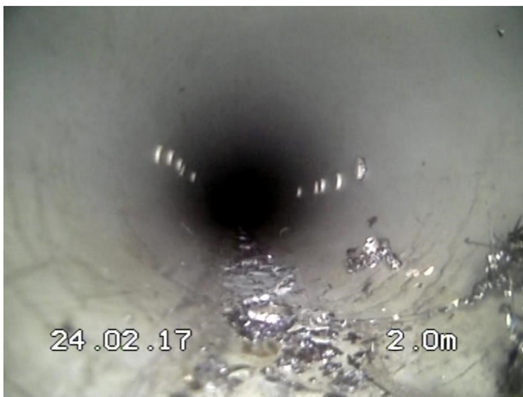
Figure 42: Right-hand outer wing, lower spar IV with swarf. Photograph provided by Ju-Air.
