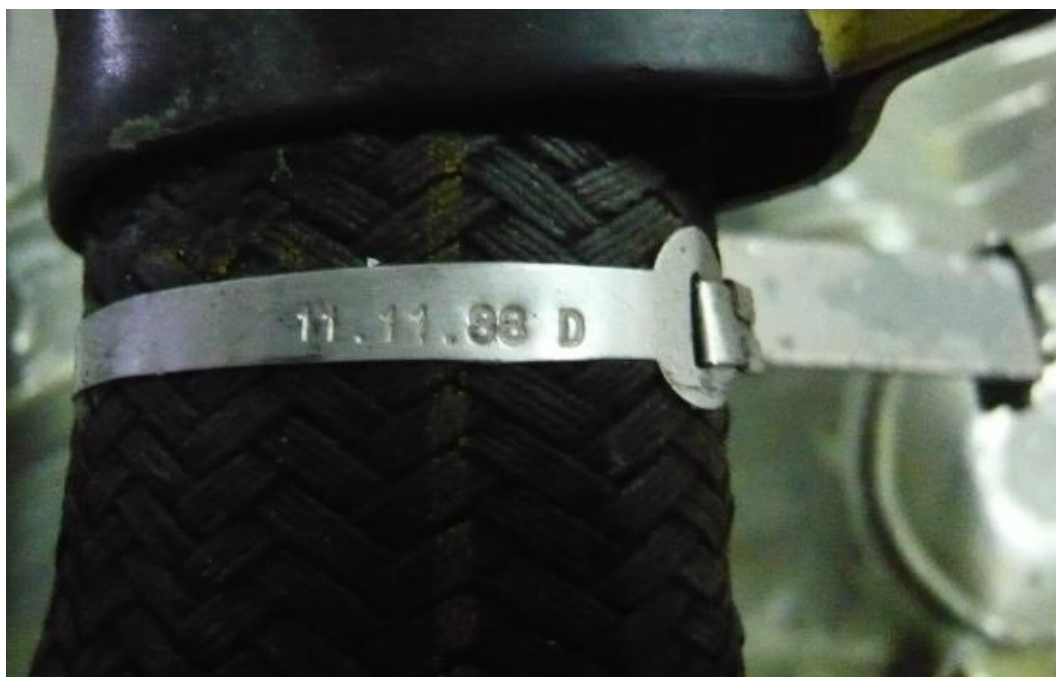
Figure 31: Hardened fuel line dated 11 November 1988.
