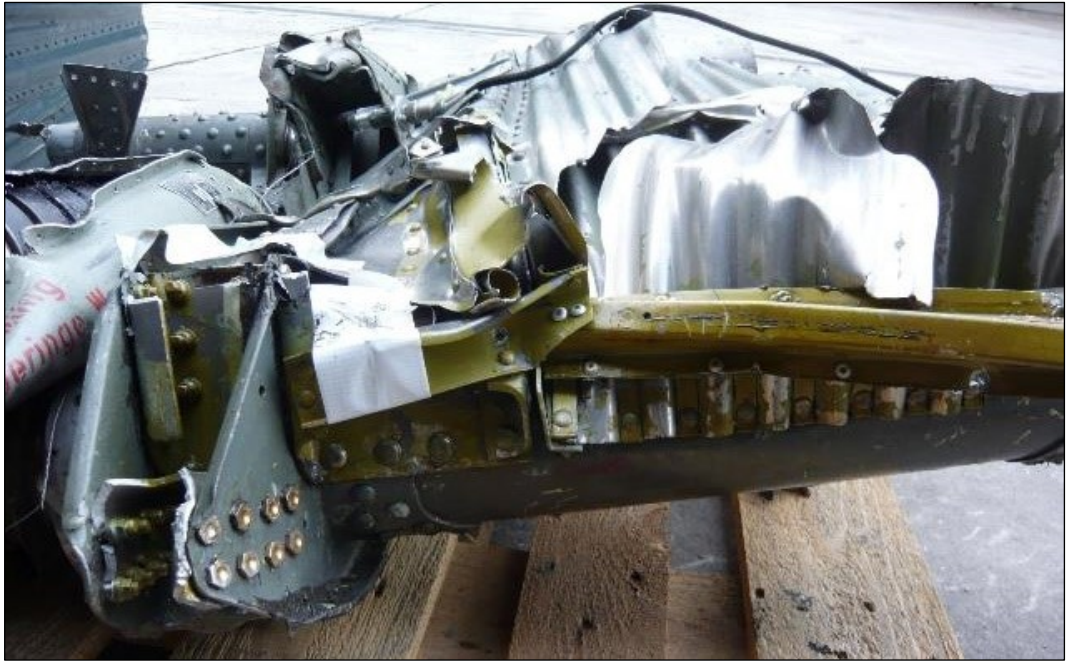
Figure 11: Repairs carried out in the centre wing, apparent by the greenish-yellow structural parts and the golden yellow connecting elements.
