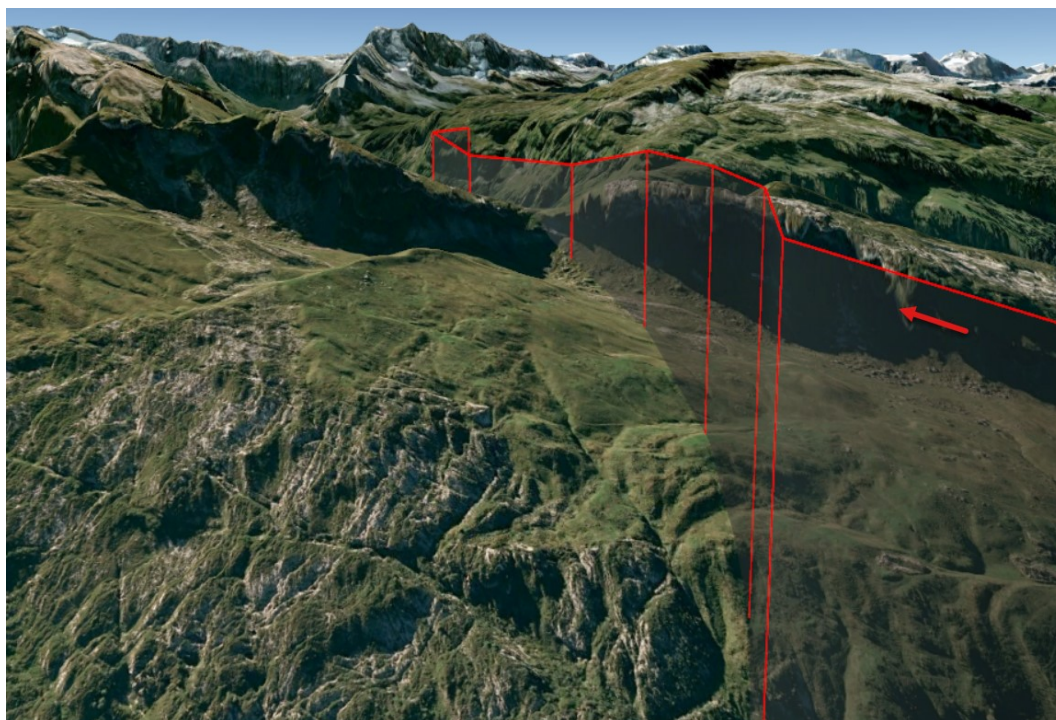
Figure 75: Descending overflight at almost 90 degrees to the terrain feature at an altitude of 1,901 m AMSL with a height of 78 m above ground directly below the radar flight path and 81 m above ground with respect to the lowest point of the terrain profile. Shown on Google Earth.
