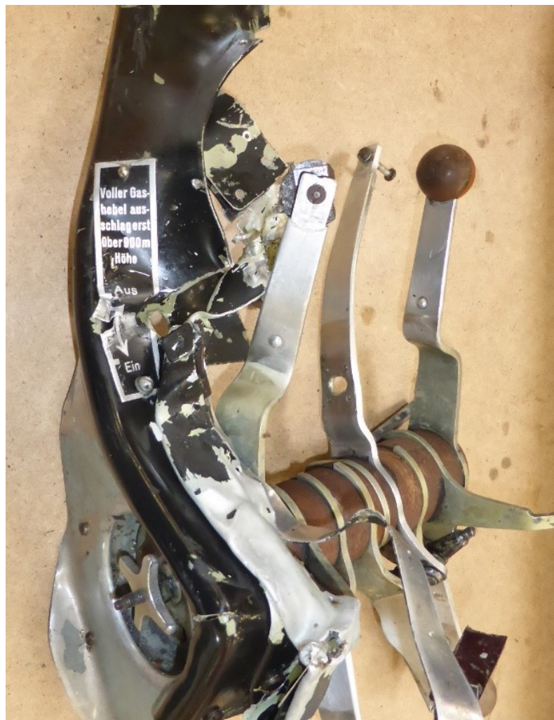
Figure 86: Deformed main throttle levers.
