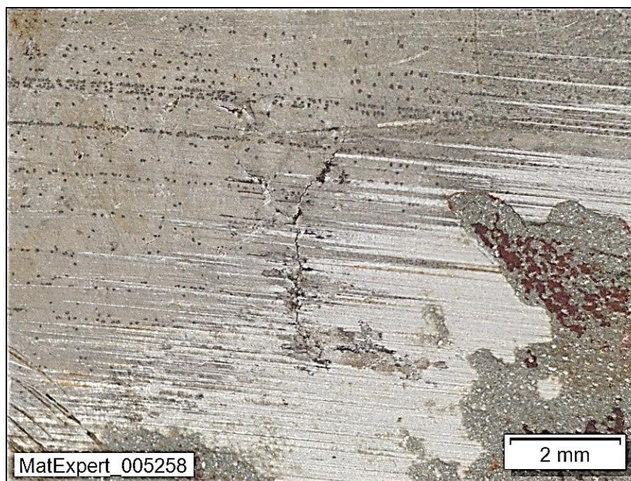
Figure 28: Area around joint 15 – brittle cracking, partially intergranular.
