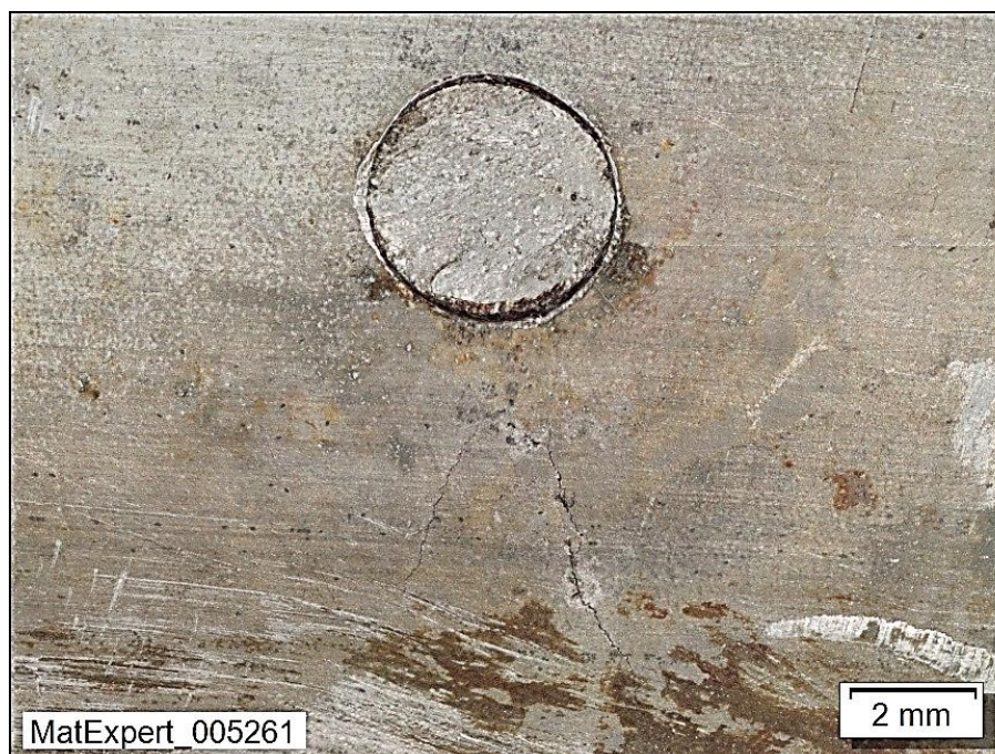
Figure 29: Area around joint 15 – brittle cracking, partially intergranular.
