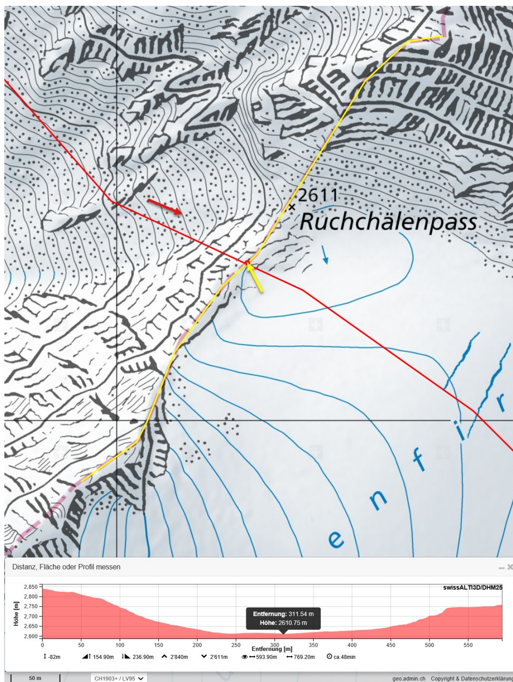
Figure 15: Depiction of the radar flight path (red line) in the direction of flight (red arrow) and the terrain profile (yellow line) with a height of 122 m above ground (2,610 m AMSL) at the lowest point of the terrain profile (yellow arrow). Source of the base map: Swiss Federal Office of Topography.
