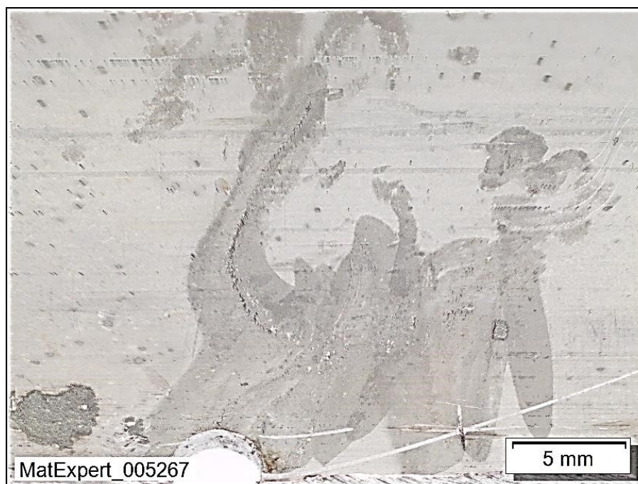
Figure 30: Area around joint 15 – crack-like surface condition.
