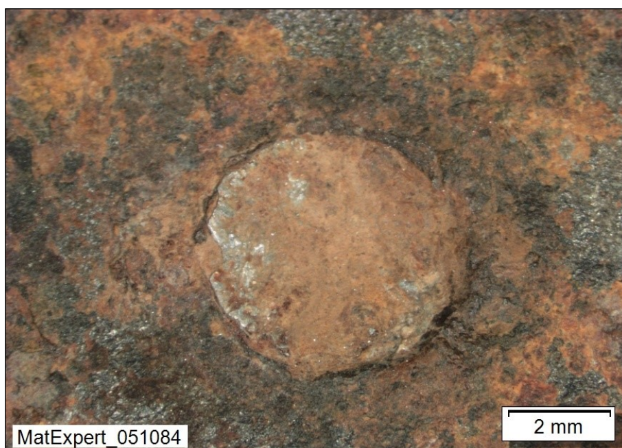
Figure 21: Close-up – broken rivet N4 with severe corrosion.
