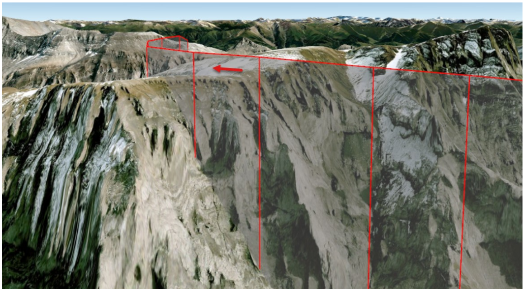
Figure 17: Horizontal overflight at 90 degrees to the crest of the mountain ridge at an altitude of 2,982 m AMSL with a height of 88 m above ground directly below the radar flight path and 96 m above ground with respect to the lowest point of the terrain profile. Shown on Google Earth.
