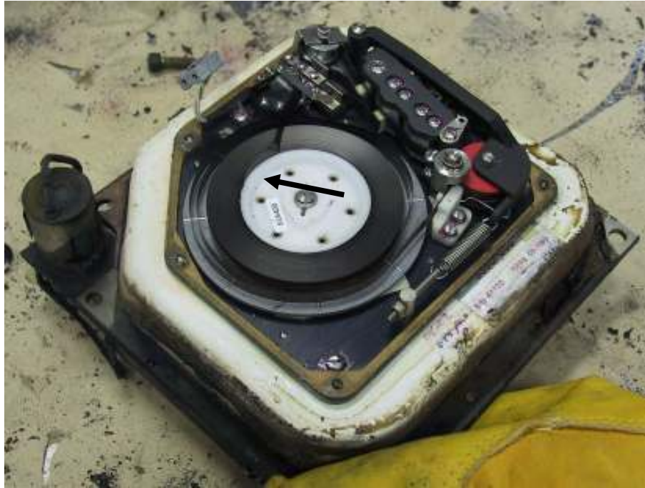
Figure B-5: Recording tape in tape transport; note slight damage to tape at centre of spool.
