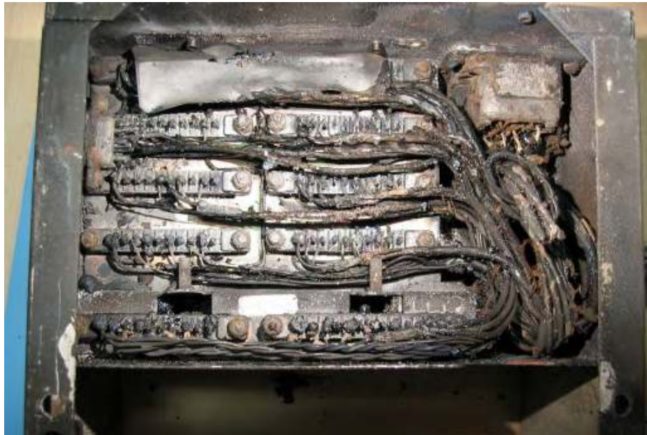
Figure B-21: VH-TFU CVR printed circuit card assembly wiring
