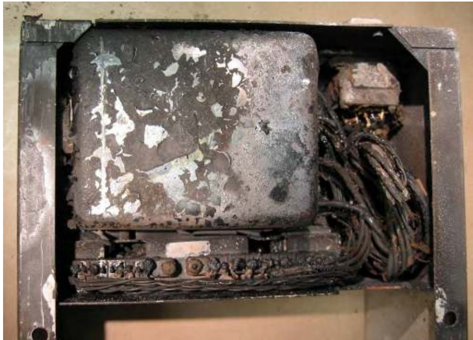
Figure B-27: VH-TFU CVR inverter assembly
