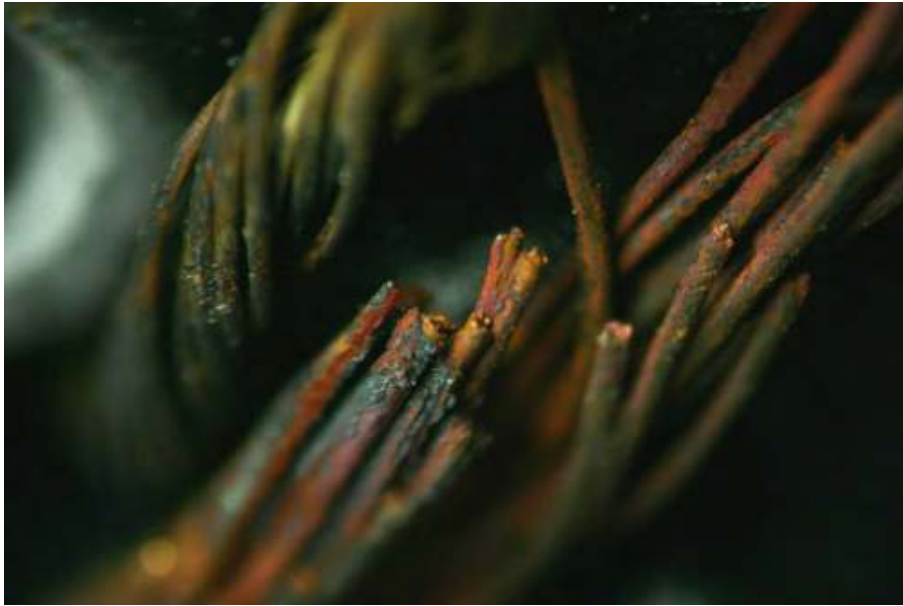
Figure B-18: Highly magnified electron microscope image of wire strands connected to pin 9 of the aircraft interface connector
