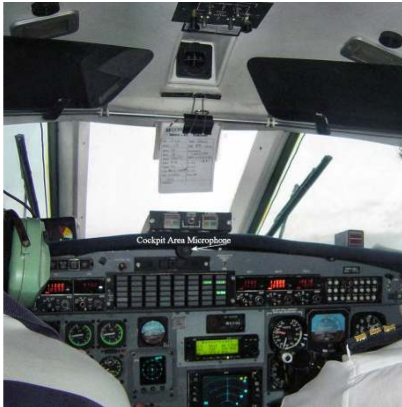
Figure B-8: Photograph of VH-TFU instrument panel showing location of cockpit area microphone.
