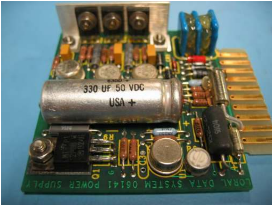
Figure B-24: Serviceable power supply card
