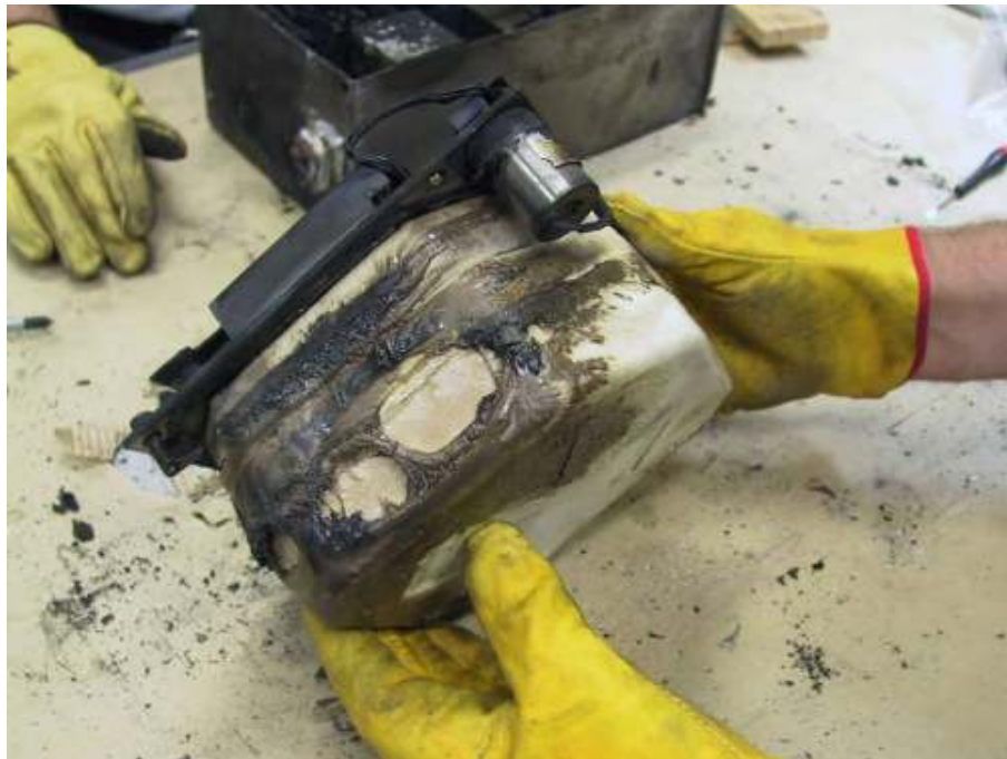
Figure B-4: Crash protected module with armouring removed. Heat damage to the fire protection can be seen.
