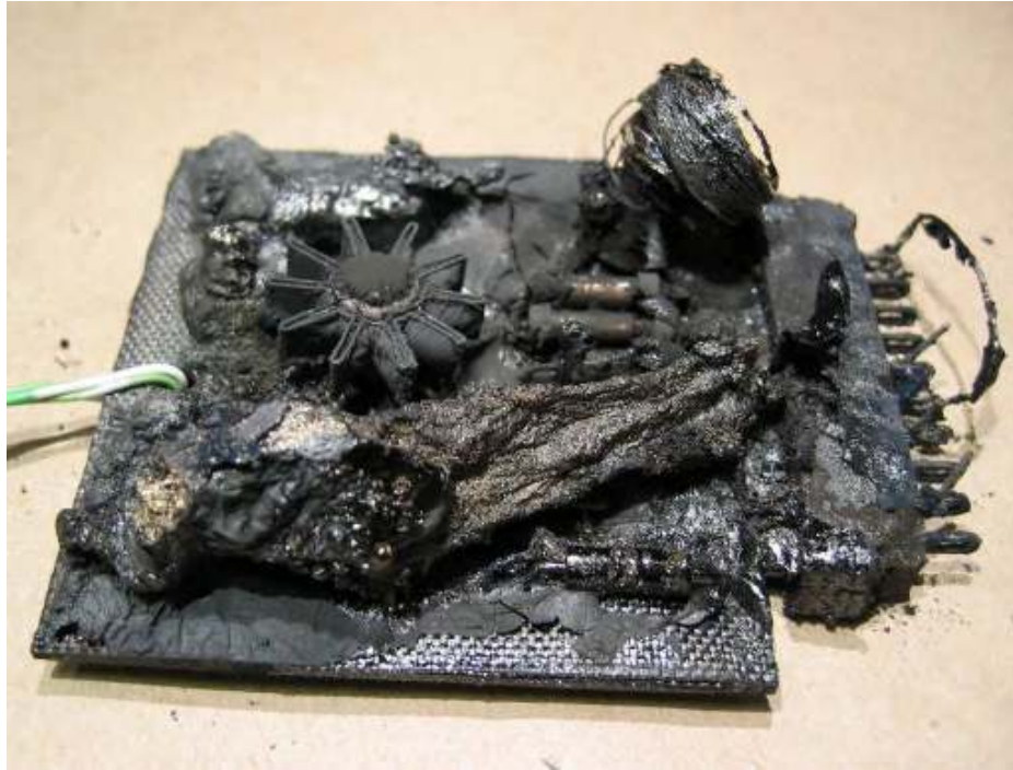
Figure B-25: VH-TFU bias oscillator assembly
